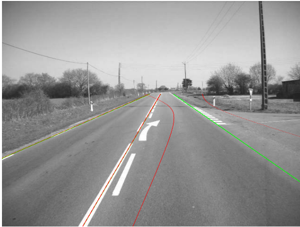
Fig. 2. Detected lane-markings (in green) and uncertainty about curve position (in red)
